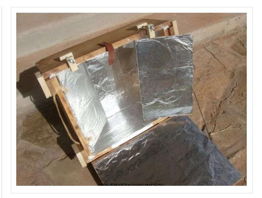
Next, I made a couple of small reflectors from cardboard to fit at 45 degree angle inside the box. These are loose and can be removed to accommodate different sized cooking vessels, etc.
