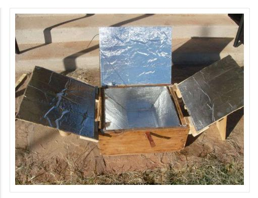
In this photo I have it set up like a typical box cooker and this will work best in the summer when the sun is higher in the sky. Since the sun is more intense when straight overhead, you may not even need the side reflectors.
