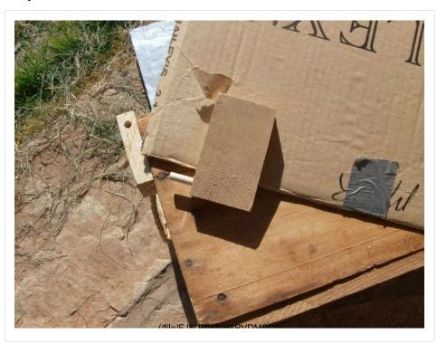
Then I made a couple of prototype (I may make these from ¼ inch plywood later) side reflectors from cardboard. These are approximately 16 inches by 20 inches.
